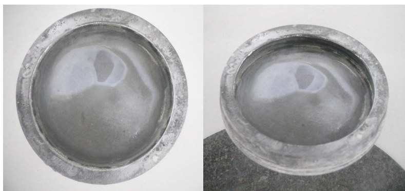
Figure 6. X65 sample at the end of 5 days exposure to \text{H}_2\text{SO}_4 (95 wt.%) in dense phase \text{CO}_2 .
